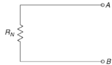
Fig. 3.256 Norton's equivalent network
